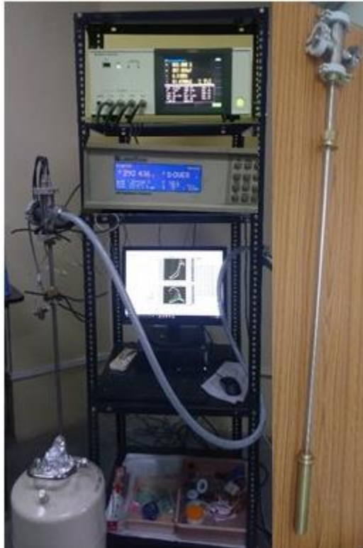
Fig 5. Dielectric measurement setup with cryo facility.
