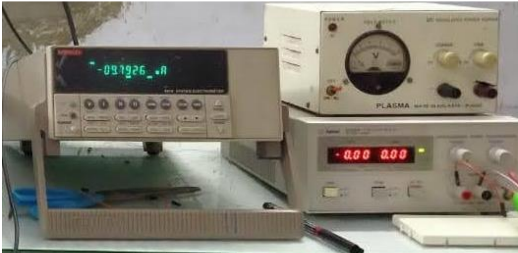
Fig 4. I-V characterization unit
